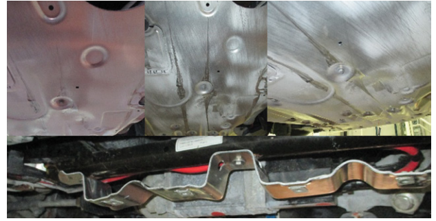
Figure 6. Scratches of the Underbody after the Physical Testing
